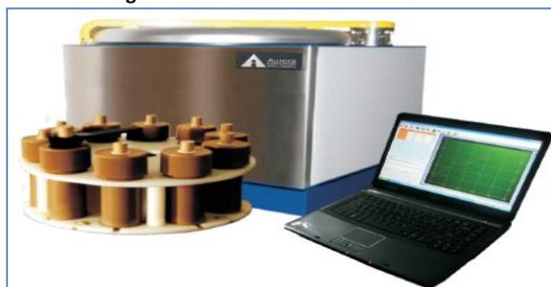
**Fig. 6:** Make-Metrohm, Switzerland, Model – 797VA Trace Metal Analyzer (Application Bulletin 96/5e by Metrohm India Limited) <sup>4</sup>
